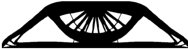
FIGURE 11. Experiment 3: Obtained result for the constrained case with \alpha = 0 , \kappa = 1.0 and M = 0.5 |\mathcal{D}| .
