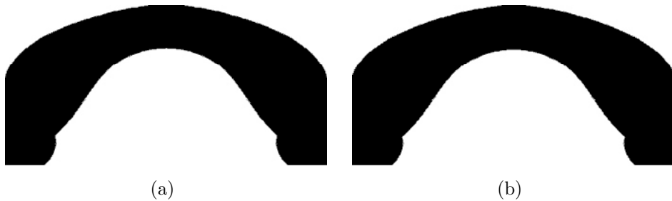
FIGURE 5. Experiment 1: Obtained results for the unconstrained case (a) with \alpha = 0.245 and for the constrained case (b) with \alpha = 2.3 and M = 0.5 |\mathcal{D}| .
