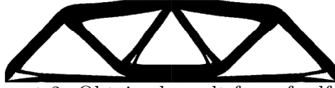
FIGURE 9. Experiment 2: Obtained result free of self-weight loading ( b = 0 ), with \alpha = 0 , \kappa = 1 and M = 0.4 |\mathcal{D}| .
