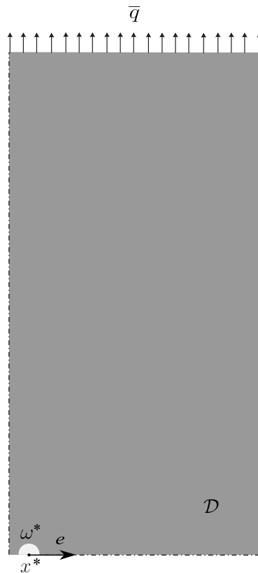
FIGURE 5. Cracked bar. Geometry and boundary conditions.
