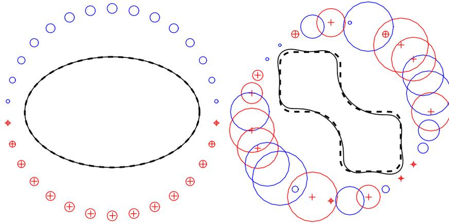
FIGURE 4. Examples 3 and 4, solutions found when considering  $m = 30$  electric currents arranged in circles of radius  $R = 1.5$  and  $R = 3.0$ , respectively.
