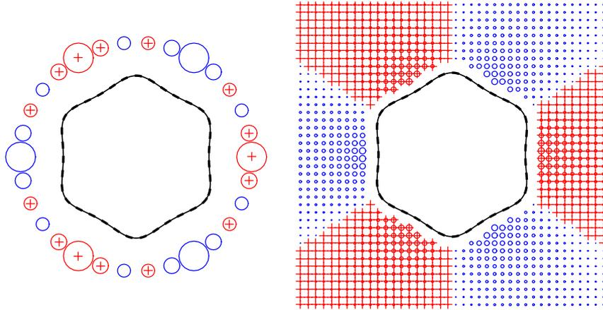
FIGURE 1. Example 1, solutions found when considering  $m = 30$  electric currents arranged in a circle of radius  $R = 1.5$  and  $m = 1188$  inductors arranged in a square regular grid. Dashed line: target shape, thin solid line: equilibrium shape for the currents found. Currents are indicated by a circle with area proportional to the current intensity, the positive currents are indicated with a plus sign.
