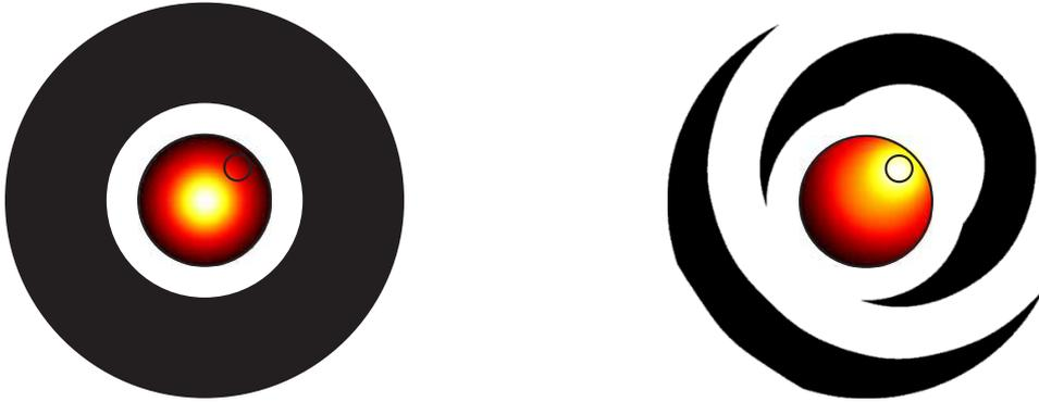
FIGURE 11. Example 1B: Experiment conducted with the wavenumber  $k = 20$ . On the left, is shown the initial configuration of the antenna  $\omega$  and initial temperature distribution in the body  $\mathcal{B}$ . On the right, is shown the final configuration of the antenna  $\omega$  and the final temperature distribution in the body  $\mathcal{B}$ , obtained after 5 iterations.
