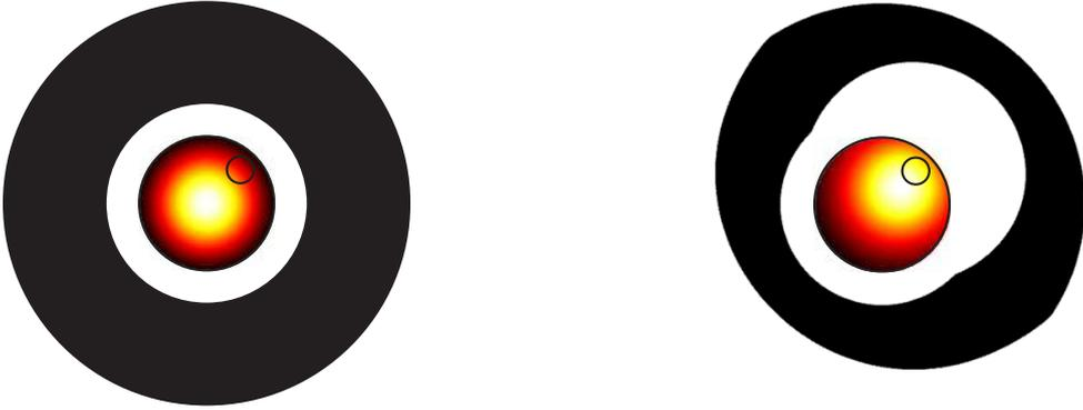
FIGURE 9. Example 1B: Experiment conducted with the wavenumber  $k = 12$ . On the left, is shown the initial configuration of the antenna  $\omega$  and initial temperature distribution in the body  $\mathcal{B}$ . On the right, is shown the final configuration of the antenna  $\omega$  and the final temperature distribution in the body  $\mathcal{B}$ , obtained after 4 iterations.
