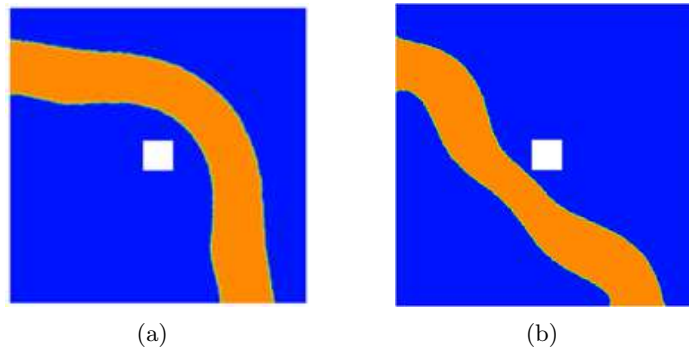
FIGURE 9. Example 3. Final topologies for obstacle problem: fluid initialization (a) and solid initialization (b).
