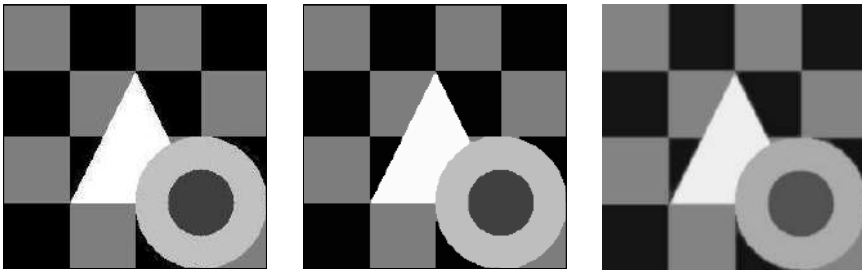
FIGURE 7. Greylevel image denoising with L^2 norm: original image (left, 240 \times 240 pixels), solution with 5 labels and \alpha = 10^{-3}\sqrt{n} (middle), solution taken from [28] (right).
