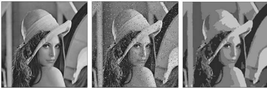
FIGURE 2. Greylevel image classification, from left to right. First: original picture ( 390 \times 390 pixels). Second: damaged image with salt and pepper noise. Third: unsupervised solution for \alpha = 4 \cdot 10^{-4} \sqrt{n} . TV-model with H = L^1 , A = I and 4 levels of grey.
