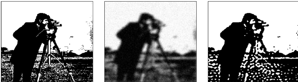
FIGURE 15. Deblurring and denoising: original image (left, 257 \times 257 pixels), damaged image with blur and noise effects (middle), reconstructed image for \alpha = 2 \cdot 10^{-4} \sqrt{n} (right).
