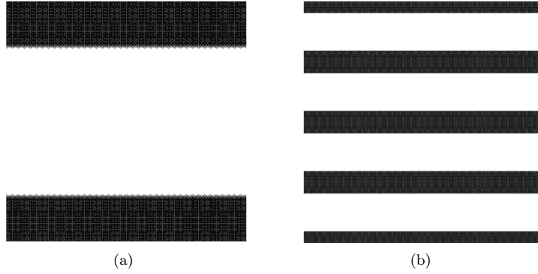
FIGURE 4. Horizontal rigidity maximization: (a) Optimum RVE topology, and; (b) Periodic microstructure.
